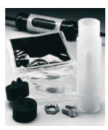
The Scotchcast 3832 Buried Service Wire Splice Kit will accommodate inline and butt splices of up to five-pair filled or unfilled service wire. One "A" size bag of 4403 encapsulant and a split bolt are provided with the kit. Once the compound has been poured, an outer tube is rotated over the barrel opening to seal the unit, requiring no waiting for the compound to cure before the kit is buried.
