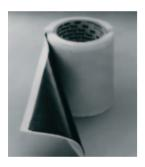
VM Tape seals out moisture and protects against corrosion without the need for heating tools. Two tapes in one (vinyl and mastic) VM is especially designed for cable sheath repair, splice case and load coil case protection, auxiliary closure and cable reel end sealing, drop wire insulating, conduit repair and protection of CATV
