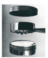
Protecting a buried service wire splice is now easier than ever with the SLiC Buried Service Wire Kit. The BSW kit is a three-part, rigid body closure that self-encapsulates two and five-pair buried service wire. It has a built-in bonding system that bonds the buried service wire shield as the splice is put together and contains a revolutionary new sealant.
