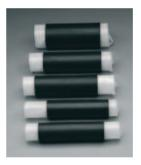
Pull 'N' Shrink Tubing is an openended tubular rubber sleeve (of high stretch EPDM rubber) which has been factory expanded and assembled into a removable hollow core. To use, the core mounted tubing is correctly positioned over a coaxial cable connector and then shrunk in place by pulling out the specially designed core allowing elastic recovery of the tube. This
