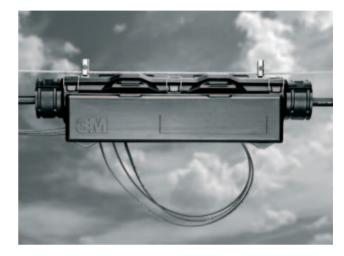
can be extended while maintaining their initial strength. The SLiC aerial closure does not require taping, bricking or any special labour-intensive practices. The end seals assure a snug fit on cables and eliminate the need for a drip collar. Sealing collars or tape are not required when using the SLiC closure.
